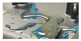
For harsh chemical environments, the Goliath is available with an optional PVDF coating. PVDF is a type of thermoplastic fluoropolymer derived from vinylidene fluoride. It is known for its high chemical resistance, UV resistance, and excellent weatherability.
